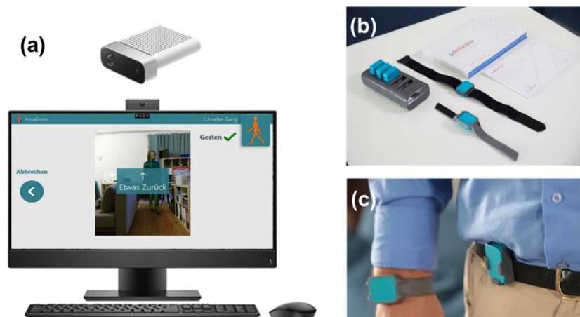
Figure 1. Overview of the sensor system and camera system used in the study. The camera system (a) consists of an all-in-one PC with the Motognosis Amsa software installed and a Microsoft Azure Kinect depth camera. The monitor shows prerecorded videos to instruct for the motoric tests. The sensor system (PDMonitor) consists of a smartbox and 5 sensors (b), which are attached to each limb and the waist (c) and worn for 6 days in a row. Image sources: Motognosis GmbH (a) and PD neurotechnology Ltd. (b,c), used with permission.
